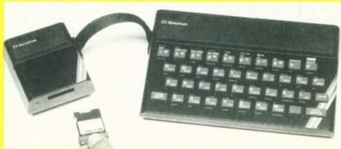
A Microdrive connected, showing how the cartridge is inserted
